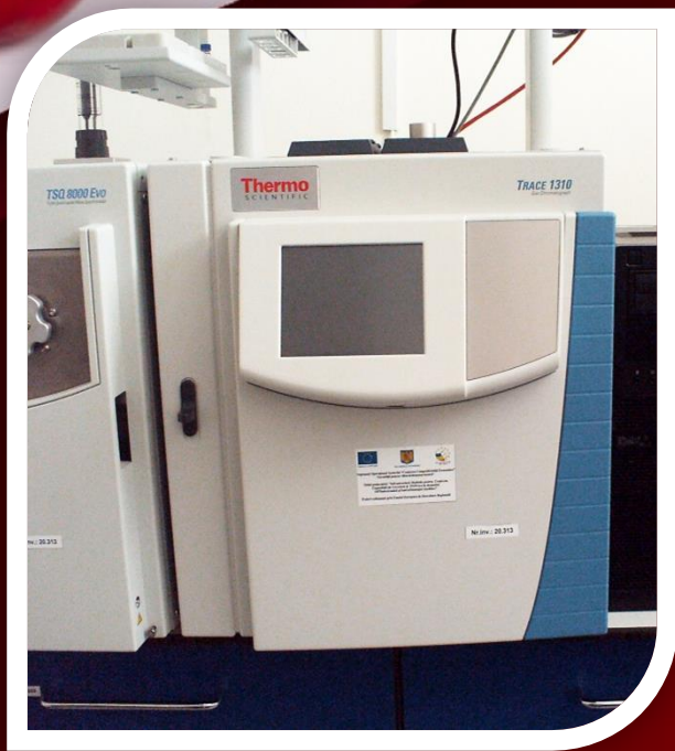
Cromatograf de gaze complet automatizat GC TRACE™ 1310 Thermo Scientific™
